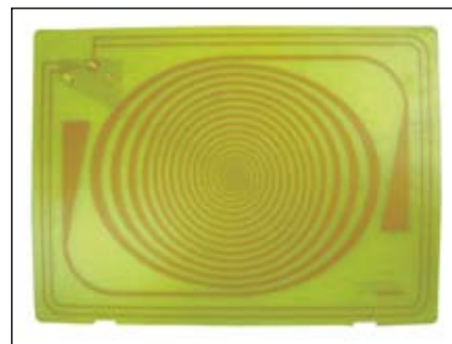
▲ Fig. 4 A bi-directional spiral antenna.
