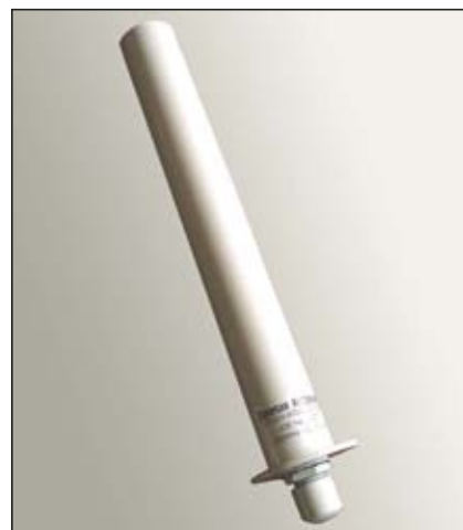
▲ Fig. 8 A bi-conical antenna.
